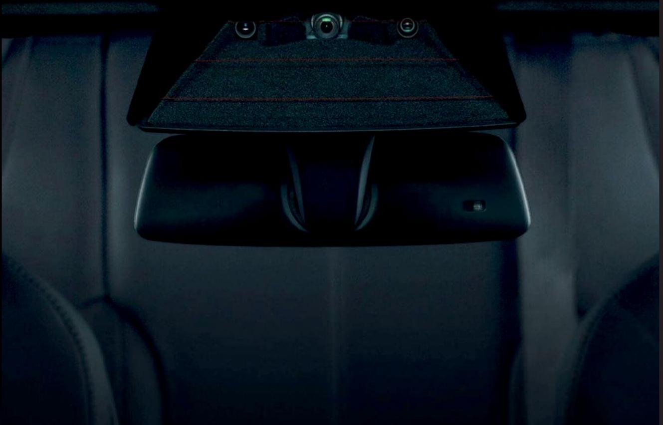
**While many ADAS systems fuse data from multiple sensor technologies (camera, radar, LiDAR etc), vision is increasingly likely to act as the mainstream solution for single sensor implementations. These feature front, side and rear view cameras for detecting traffic signs, objects, pedestrians and tracking the vehicle's lane position.**
