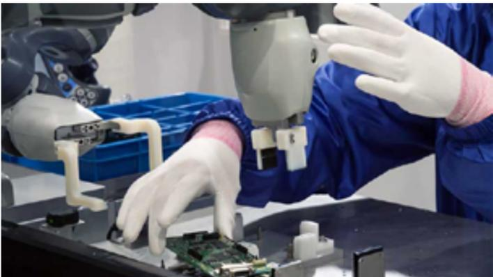
Not too long ago, robots in factories knew their place – behind safety cages, well out of harm's way. But that has changed. Now, a new breed of collaborative robots (cobots), comprising a suite of positional sensors along with connectivity, has been developed to work safely alongside humans, increasing the flexibility of the production line and boosting productivity.
