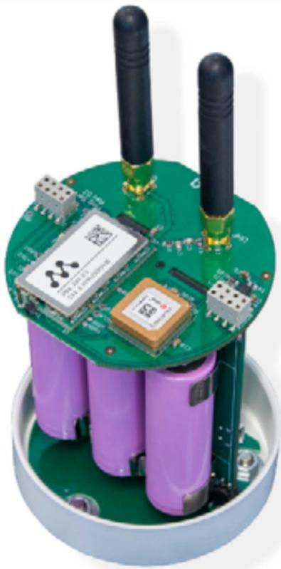
The solar-powered, satellite-connected sensors actively listen to the turbine blades' acoustic signature to detect the development of pitting or cracks, caused by lightning strikes or hail. As such issues begin to develop, they can be monitored and targeted for maintenance remotely, rather than requiring highly trained teams to tour windfarms and conduct routine testing.
